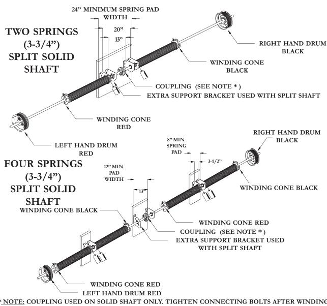
\*NOTE: COUPLING USED ON SOLID SHAFT ONLY. TIGHTEN CONNECTING BOLTS AFTER WINDING SPRINGS. PG. 9
